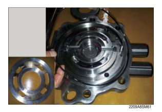
② Using a torque wrench, disassemble relief valve (30) from valve casing (23).
