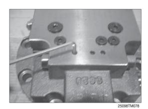
(3) Assemble the spool (47), parallel pin (50), spring seat (49) and spring (51) into the rear cover (34) and tighten both side of the plug (48) and connector (52) into the rear cover (34).
