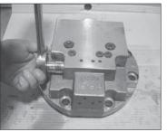
(4) Assemble the relief valve (42, 2EA) into rear cover (34).
