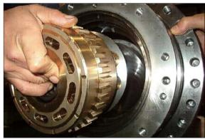
11) Assemble friction plate (19) and plate (20) into shaft casing (1) respectively, prepare 6 set.
