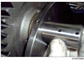
(3) Install No.1 pin (91-5) into No.1 carrier where the holes for No.1 pin (91-5) are to be in line with those of No.1 carrier, and then, install spring pins into the holes.
