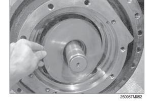
(10) Disassemble the steel ball (15) and swash piston (6) from the casing.
